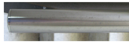
Fig. 3: Cleaned & protected surface
